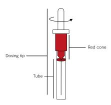
2. Remove the dosing tip from the transport tube by pulling it upwards.
